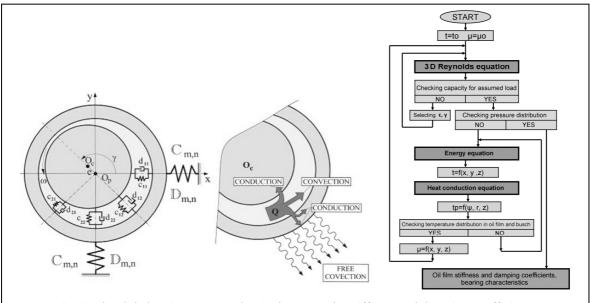
Fig. 3. The slide bearing as a mechanical system: the stiffness and damping coefficients, thermal flux, the algorithm of the slide bearing's properties' calculation
