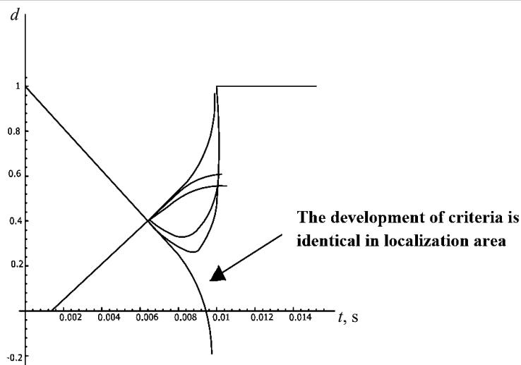
Fig. 9. Damage throughout the first three elements and criteria vs. time ( $a = 1.5 \text{ mm/s}$ ).
