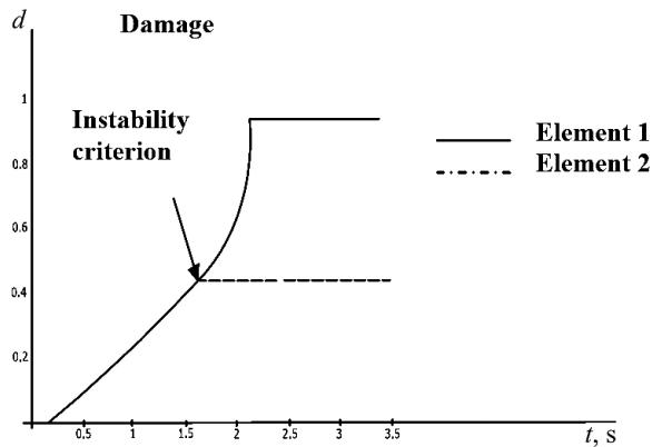
Fig. 2. Damage vs. time in the beam, localization in element 1.
