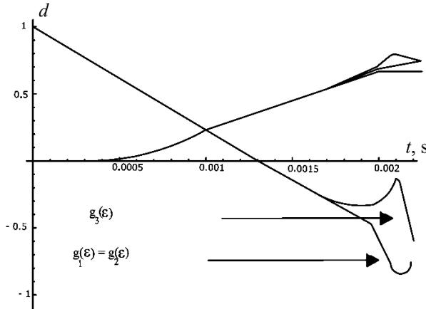
Fig. 6. Damage and criterion vs. time, localization in the elements of length  $l_1$  and  $l_2$  ( $a = 25$  mm/s).
