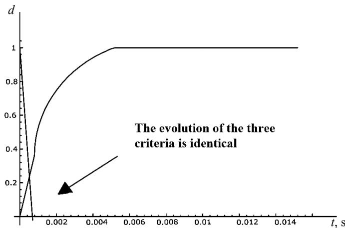
Fig. 7. Damage for all elements and criteria vs. time ( $a = 50$  mm/s).
