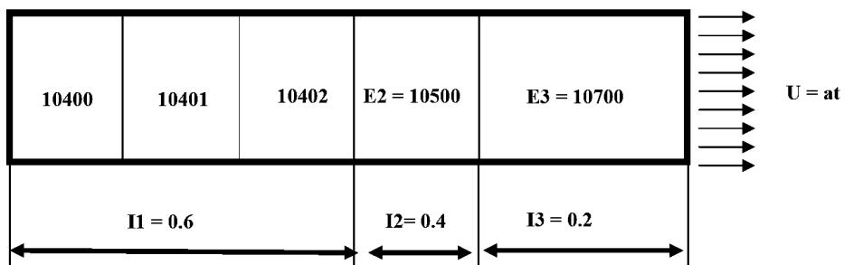
Fig. 8. Beam in tension-imposed displacement.
