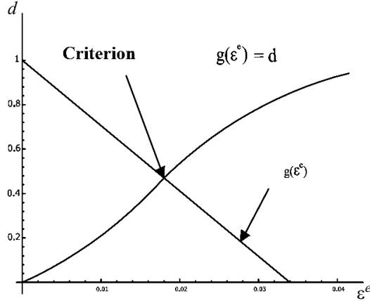
Fig. 3. Damage vs. deformation and instability criterion.
