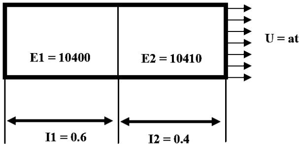
Fig. 1. Beam in tension-imposed displacement.
