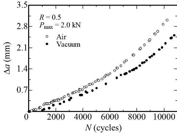
Fig. 4. The amount of crack extension  $\Delta a$  versus the number of cycles  $N$  at the load ratio  $R = 0.5$ .
