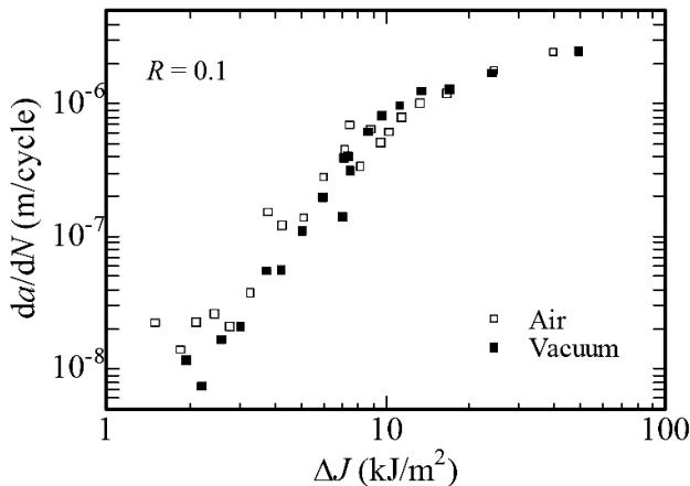
Fig. 5. Fatigue crack growth rate  $da/dN$  versus  $J$ -integral range  $\Delta J$  at the load ratio  $R = 0.1$ .
