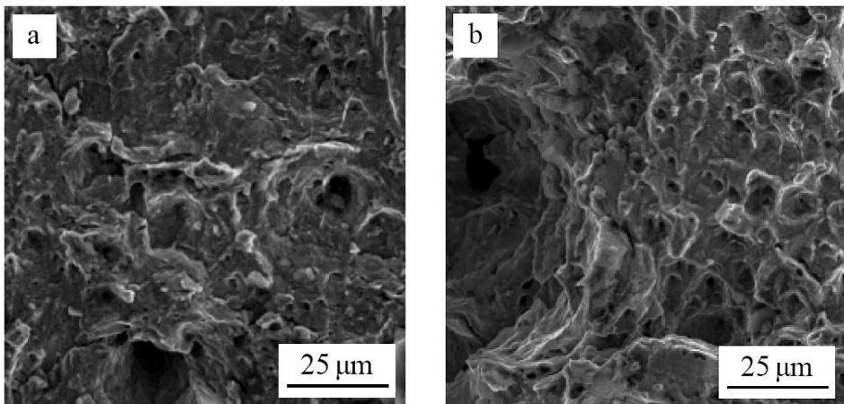
Fig. 7. SEM observations of the fracture surfaces at the load ratio  $R = 0.5$  for high  $\Delta J$  levels: (a) air; (b) vacuum (crack propagation from top to bottom).
