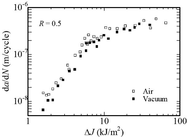
Fig. 6. Fatigue crack growth rate  $da/dN$  versus  $J$ -integral range  $\Delta J$  at the load ratio  $R = 0.5$ .
