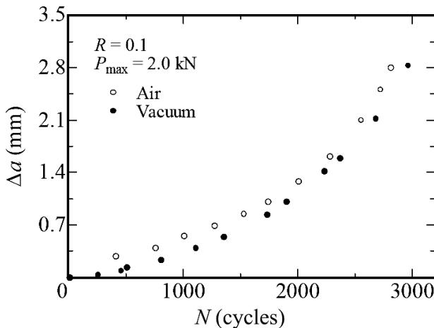
Fig. 3. The amount of crack extension  $\Delta a$  versus the number of cycles  $N$  at the load ratio  $R = 0.1$ .
