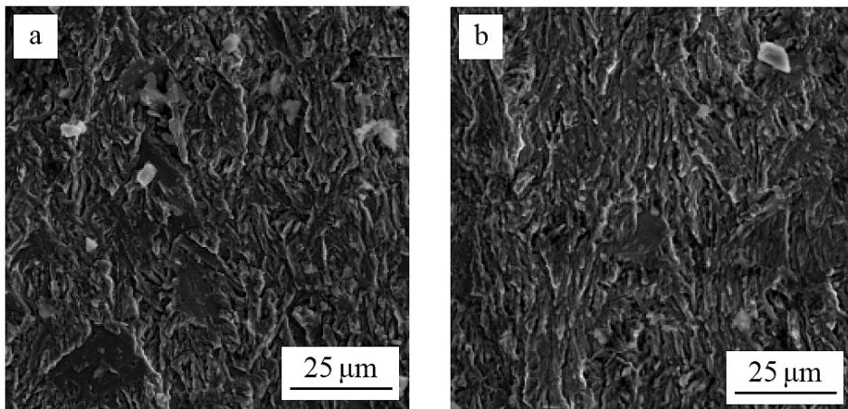
Fig. 8. SEM observations of the fracture surfaces at the load ratio  $R = 0.5$  for low  $\Delta J$  levels: (a) air; (b) vacuum (crack propagation from top to bottom).
