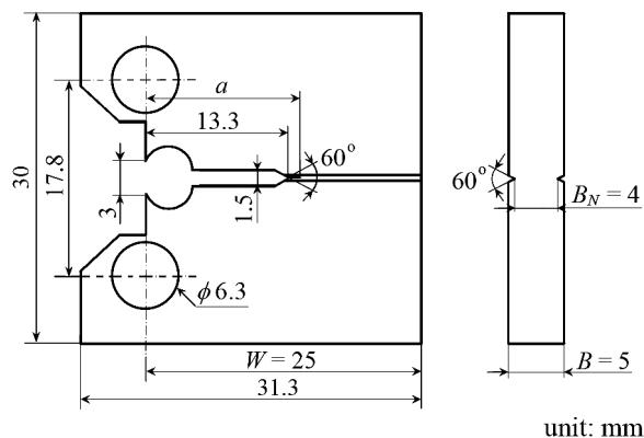
Fig. 1. Geometry and dimensions of CT specimen.
