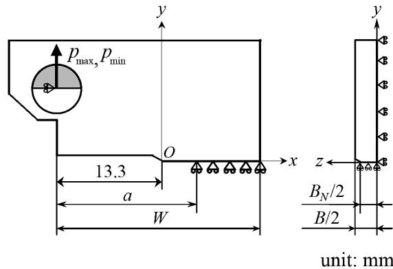
Fig. 2. Illustration of boundary conditions on the CT specimen model.
