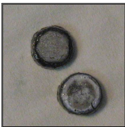
Fig. 1. Cesium ion emitters: Left up – pollux emitter after preparation, right bottom – emitter after 1.5 mA*hour operation
