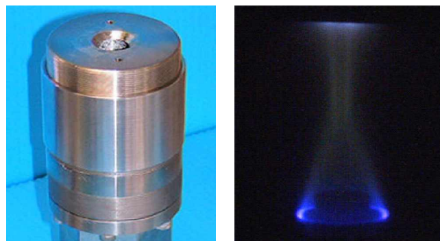
Fig. 2. The ion source used for trimming and the focused ion beam
