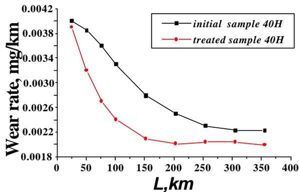
Fig. 1. Wear rate of initial and processed samples.
