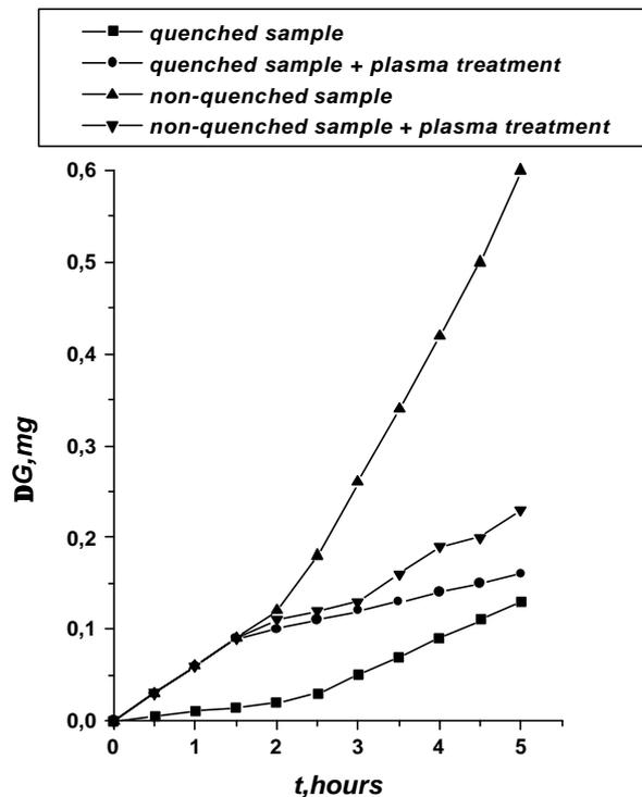
Fig. 3. Mass losses of 40H steel samples under cavitation tests.
