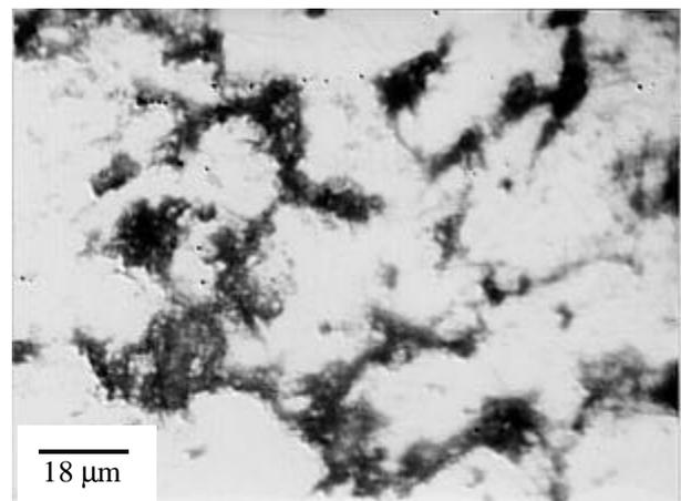
Fig.2. Sample surface after the cavitation influence.
