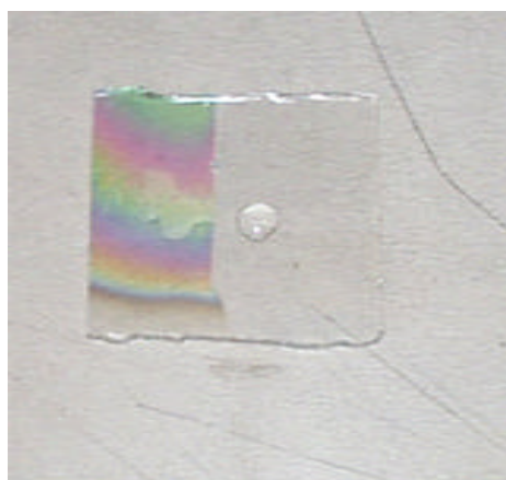
Fig.4. View of hydrophilic effect on glass; the left and right half sides are with and without \text{TiO}_2 film ( V_A = 80 V, I_D = 4 A, fluorescent lamp 15W)
