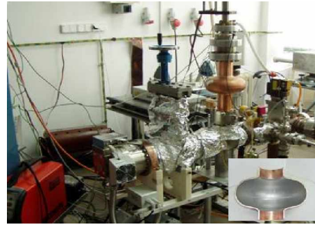
Fig.9. Modified UHV linear-arc facility constructed at IPJ for the deposition of thin super-conducting layers and the axial cut of the RF cell coated with a pure Nb-layer
