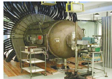
Fig.10. Large experimental chamber of PF-1000 facility
