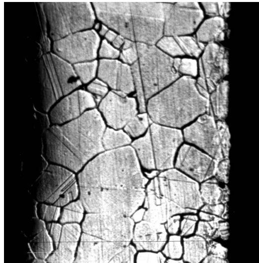
Alloy "A". Irradiation dose is 64 eV/atom
