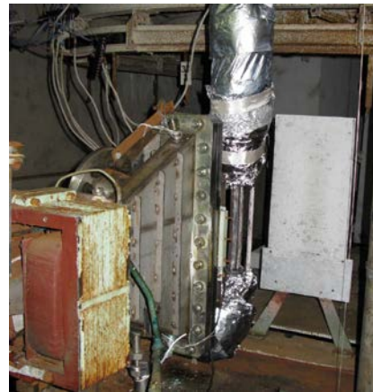
Fig. 10. Irradiated chamber with the loop and screen for electron beam monitoring
