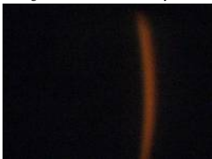
Fig. 2. Electron beam image of magnetron gun with 40 keV electron energy at the target
