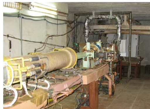
Fig. 4. LINAC LUE-10 with conveyor and supercritical water convection loop
