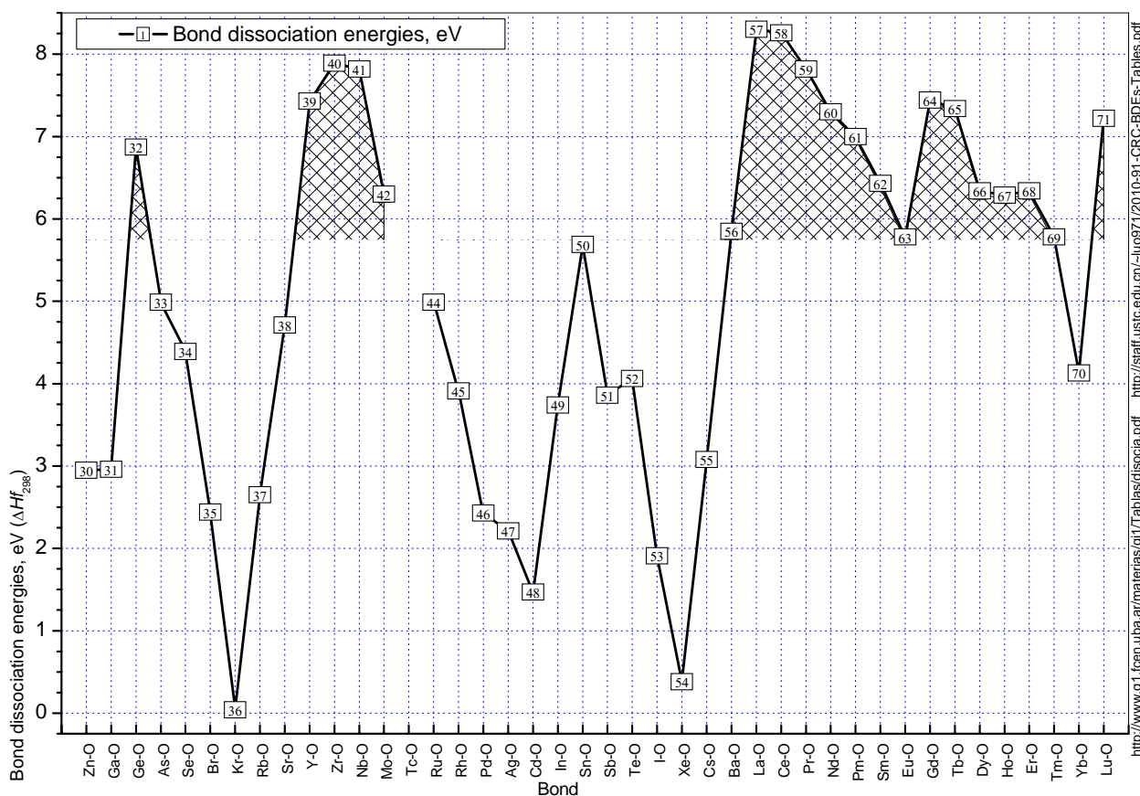
Fig. 3. Relationship of oxide dissociation energies as a function of the value of the binding energy
