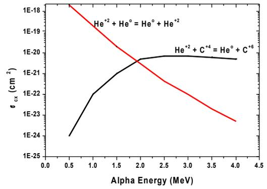
Fig 5. Cross sections of processes relevant for neutralization of alpha particles.
