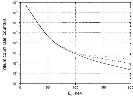
Fig.4. Energy dependence of tritium count rate for different  $He^+$  density profiles.
