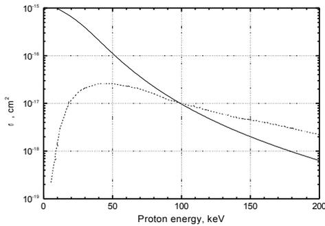
Fig.1. Proton neutralization cross-sections due to charge exchange with H atoms (solid line) and He<sup>+</sup> ions (dotted line).
