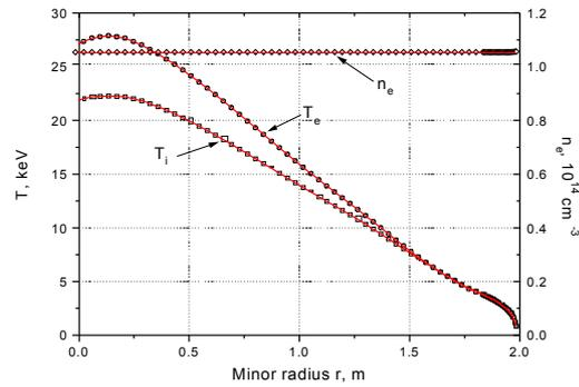
Fig. 2. ITER-FEAT temperatures and electron density versus vessel minor radius. Circles (open, closed and dot centered) are results of PRETOR code simulation for  $Q=10$  Domain. Solid curves are profiles used in D/T neutral flux simulation.
