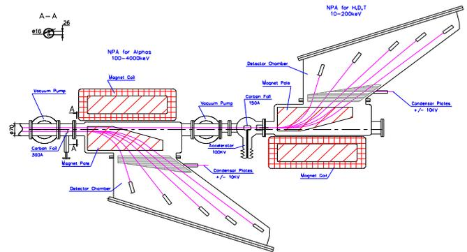
Fig. 7. The sketch of the NPA system developed for ITER.
