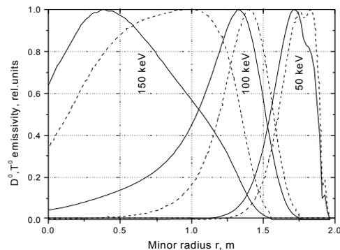
Fig.3. Emissivity functions of D<sup>0</sup> and T<sup>0</sup> atoms of different energies from ITER-FEAT standard discharge plasma. Solid lines – for D<sup>0</sup>, dashed lines – for T<sup>0</sup>.
