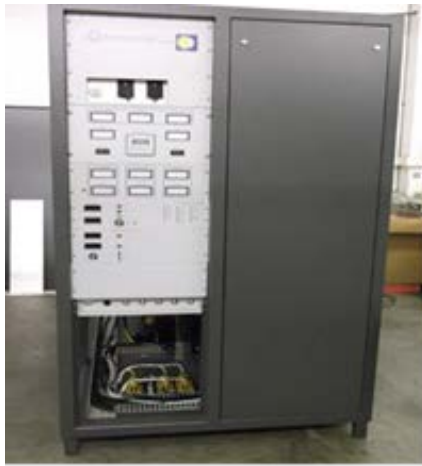
Fig. 4. The RF-power amplifier
