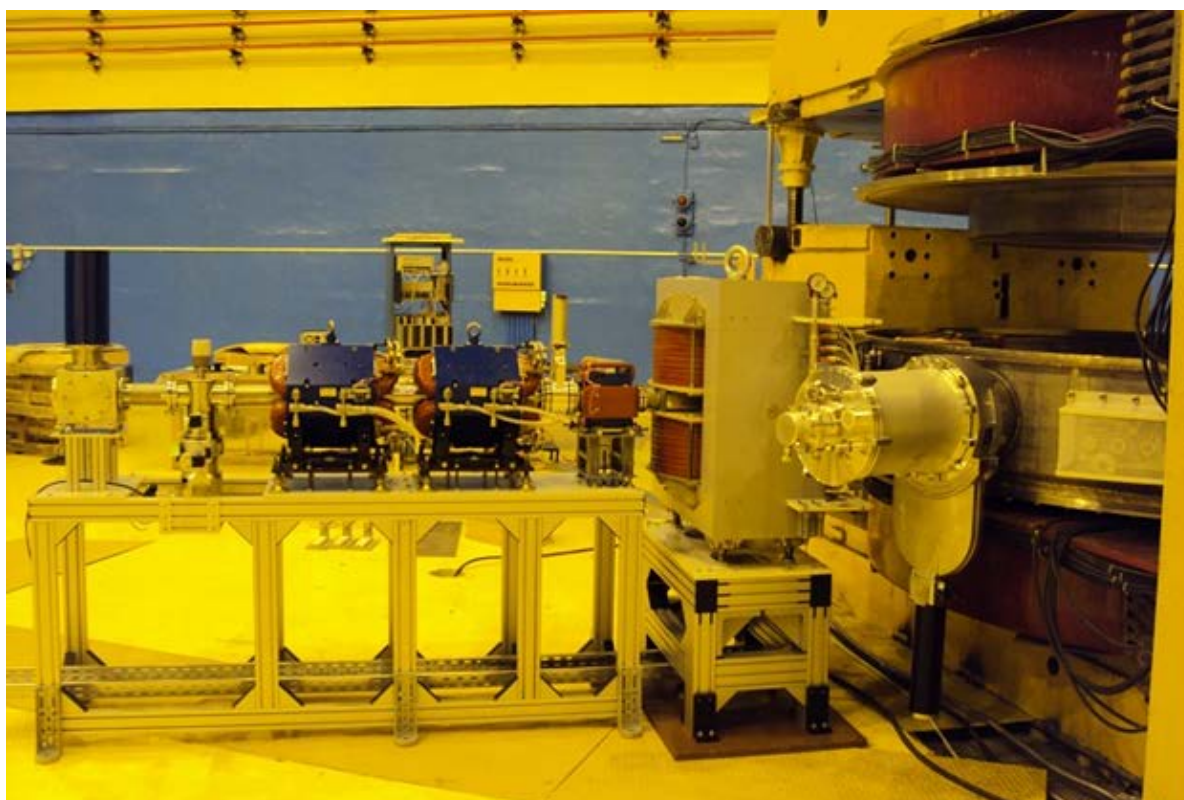
Fig. 8. The 1 st section of the beam transport system
