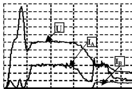
Fig.6. Oscillograms for the private case magnetron mode ( I_A – radial beam and I_B – axial beam). Horizontal - 2 \mu\text{s/div}
