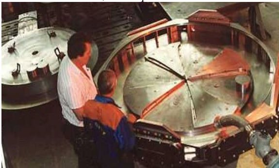
Fig.4. In foreground-bottom pole with the vacuum chamber, on the left-top pole with the cover of the vacuum chamber
