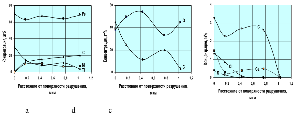
Fig.3. Content of the primary alloying elements (a, except for light and impurity ones), oxygen, carbon (b), as well as sulfur, chlorine, copper and calcium (c) against the fracture surface distance in the irradiated steel
