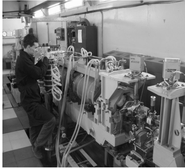
Fig. 5. Accelerating structure of the linac.
