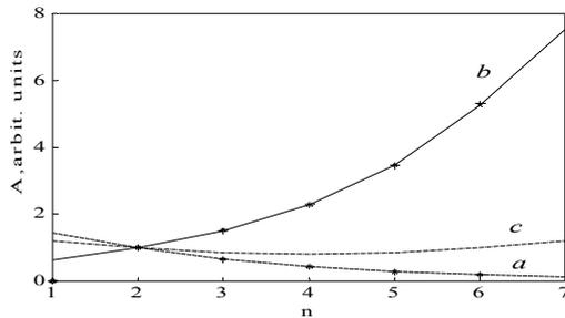
Fig. 2. Amplitude distribution in the structure consisting of 7 cavities at the frequency  $\omega=1.004\omega_\pi$ :
