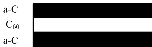
Fig. 2. "Sandwich" structure a-C/ C_{60} /a-C.
