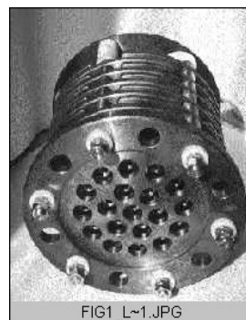
Fig.1. Model of the multiple channel system for ion beam formation
