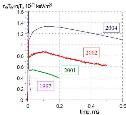
Fig. 3. Plasma pressure behavior in the GOL-3 facility. 1997-uniform magnetic field with two end mirrors,  $n_e=0.9 \cdot 10^{21} \text{ m}^{-3}$  (hydrogen); 2001-4 m corrugation from each side,  $n_e=0.3 \cdot 10^{21} \text{ m}^{-3}$  (deuterium); 2002-fully corrugated magnetic field,  $n_e=0.8 \cdot 10^{21} \text{ m}^{-3}$  (deuterium); 2004-improved heating with full corrugation,  $n_e=1.5 \cdot 10^{21} \text{ m}^{-3}$  (deuterium)
