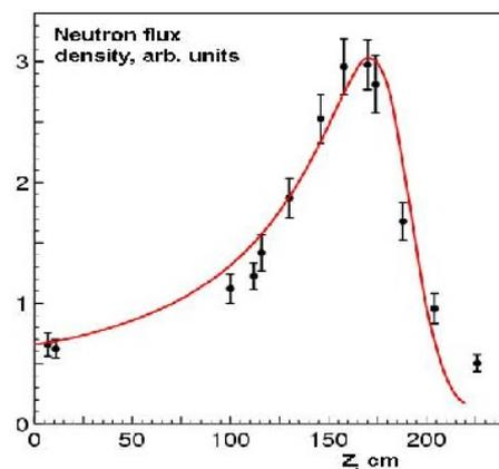
Fig.5 Axial profile of D-D neutron flux in GDT
