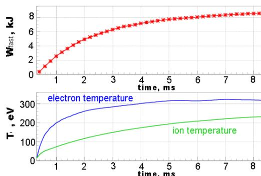
Fig.6. Temporal variation of fast ions energy content  $W_{fast}$ , electron and ion temperature in GDT-U
