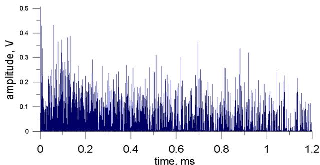
Fig. 4. Neutron radiation of plasma in GOL-3 after plasma heating by REB (duration of REB is  $8 \cdot 10^{-6} \text{ s}$ ) recorded by digital PSD stilbene detector at  $Z=4.3 \text{ m}$ . Plasma density is  $1.9 \cdot 10^{21} \text{ m}^{-3}$
