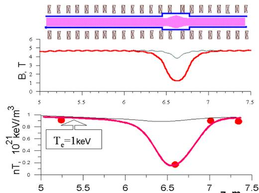
Fig.2. Direct observation of anomalously low longitudinal electron heat conductance during the process of collective relaxation of REB in plasma
