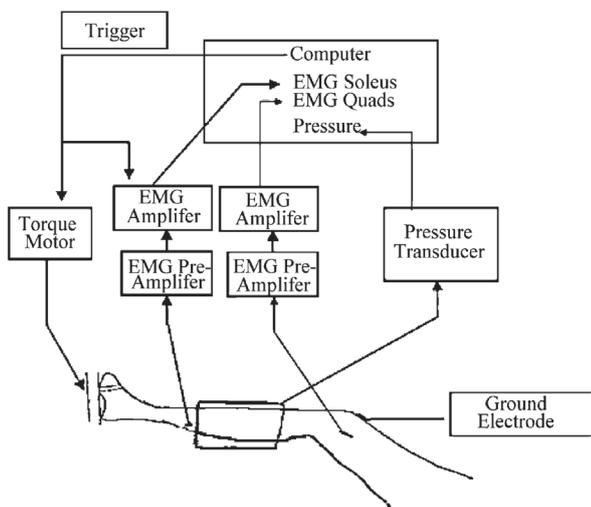
Fig. 1. Scheme of the experimental setup.
