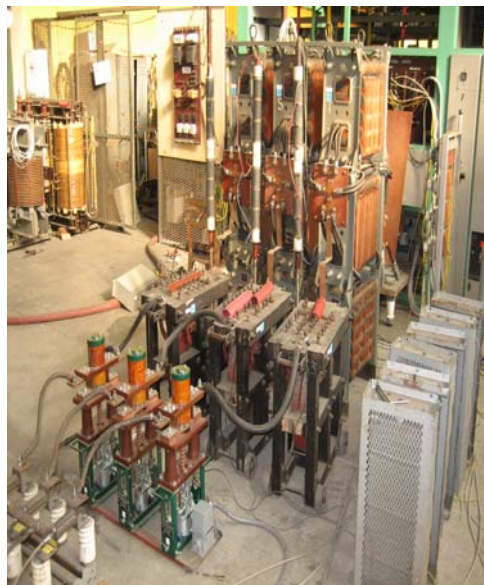
Fig. 2. Circuit diagram and view of the switching test stand: S — supply; U_{r1}, U_{r2} — voltage meters; A — auxiliary switch; R_1, X — resistive and inductive controllers; F — high power fuse; R_L — ground current limiter; D — contactor under test; I_1 — current meter; r — shunt; B — link for graduation.
