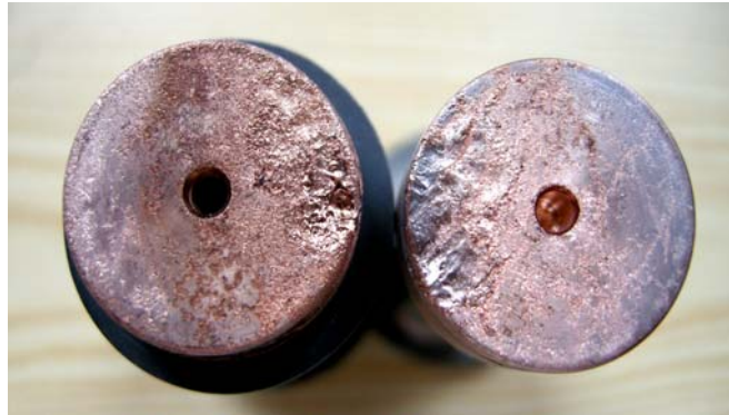
Fig. 5. View of the failed contact surface after welding.
