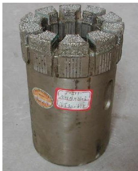
Fig.6. Electroplating Diamond bit by two-step forming manufacture technology
