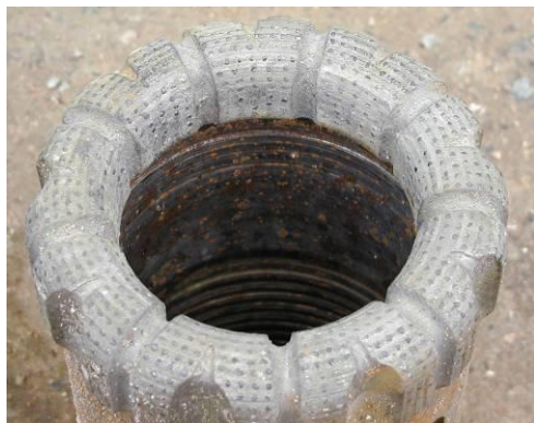
Fig.1. Wear situation of surface-insert type diamond bit
