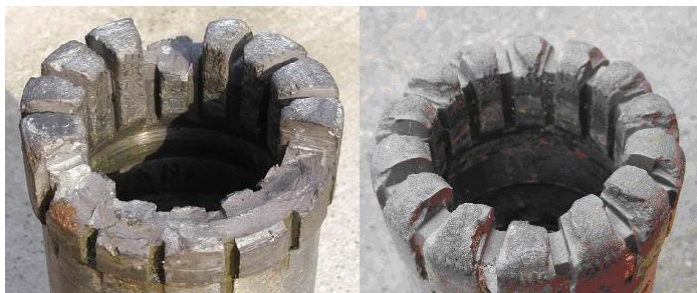
Fig.3. The collapse of the bit crown
