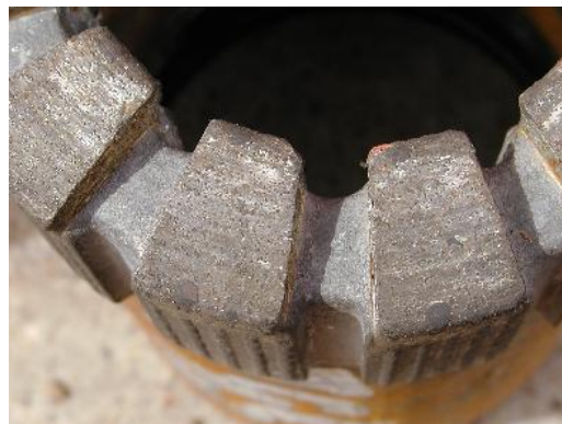
Fig.2. The edge situation of diamond under impacting action by hydro-hammer
