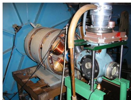
Fig. 1. System of the beam formation and transport from accelerating section output to the irradiation chamber
