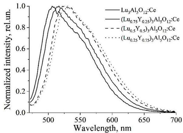
Comparison of the normalized luminescence spectra of composite scintillators based on grains  $(Lu_xY_{1-x})_3Al_5O_{12}:Ce$  (grains size 0.3...0.5 nm) with excitation of the light wavelength of 460 nm
