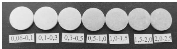
Fig. 1. Photo of polycrystalline scintillators of p -terphenyl obtained from grains of different fractions
