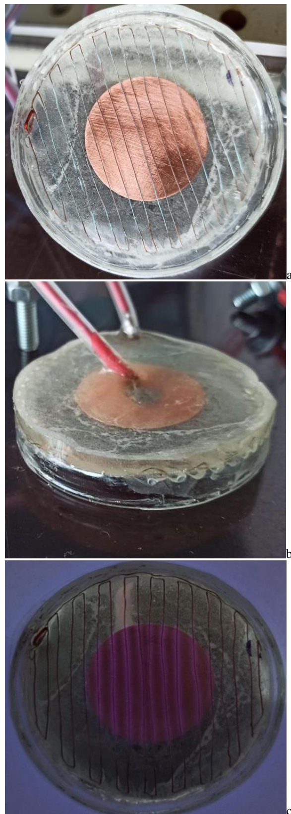
Fig. 2. Photos of DBD electrodes system designed for treating seeds before planting: lower electrode (a); upper electrode covered with epoxy resin (b); DBD during operation (c)
