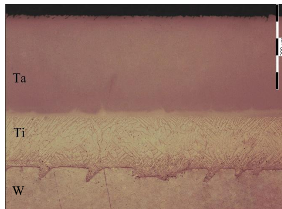
Fig. 3. The microstructure of Ta-W-Ta solid-phase junction with Ti interlayers specimen, \times 200
