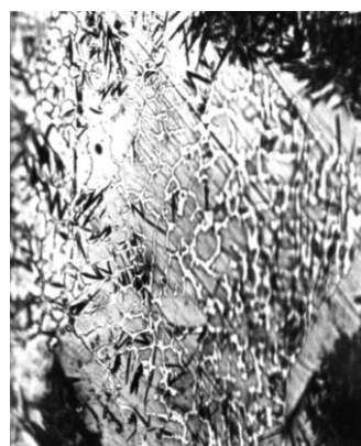
Fig. 3. Infusion zone. Structure of the high-carbon steel tempered from a melted mass, x500
