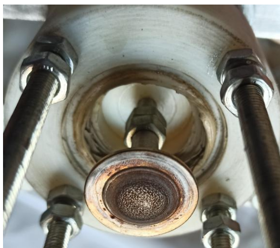
Fig. 5. Typical photo of T-shaped cathode after long-term operation
