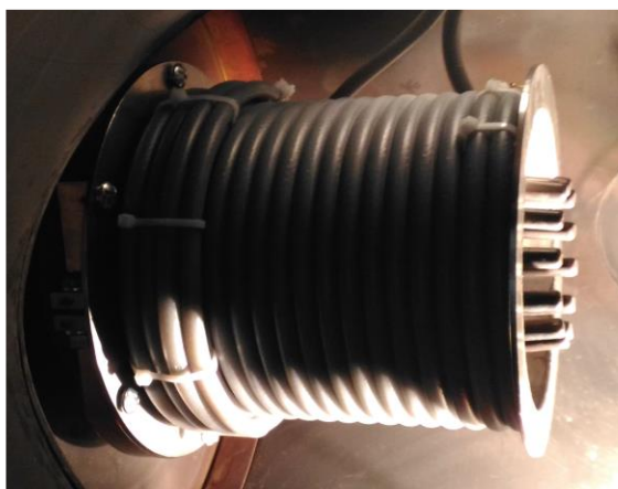
Fig. 1. MPC accelerating channel with a solenoid
