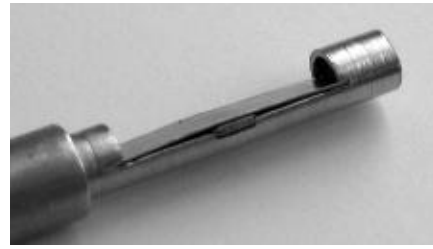
Fig. 3. The strained coupon mounted inside the IC internal sample holder with the bend adjusting screw
