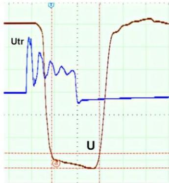
Fig. 5. Voltage pulse at the output of the forming line with overcorrection (U) 20 V/div, voltage pulse trigger (Utr) 10 V/div 2  $\mu$ S/div
