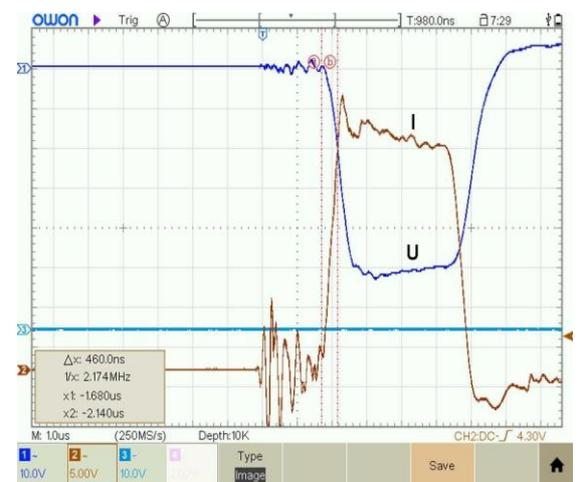
Fig. 4. Voltage (U) and current (I) pulse on the secondary winding of the pulse transformer of the technological accelerator LINAC-40:  $15 \text{ A/div}$ ,  $30 \text{ kV/div}$ ,  $1 \mu\text{s/div}$
