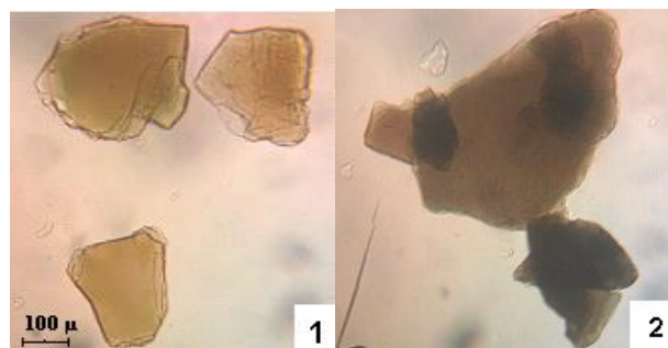
Fig. 4. Microphotographs of an immersion preparation of biotite, in transmitted light, view without an analyzer: 1 – initial biotite; 2 – after irradiation to D=10^7 Gy
