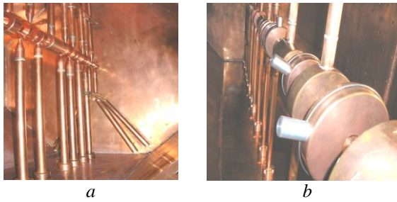
Fig. 3. Accelerating structure of helium ion linac with output energy 4 MeV: inside view (a); accelerating&focusing channel with tuning elements (b)
