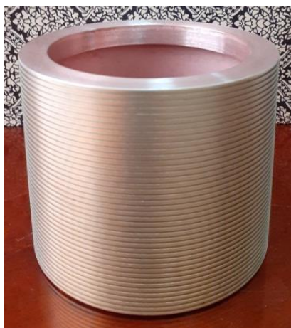
Fig. 1. A sample of a copper cathode coated with zirconium nitride and an intermediate layer of molybdenum
