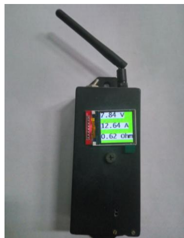
Fig. 7. Receiving module assembly
