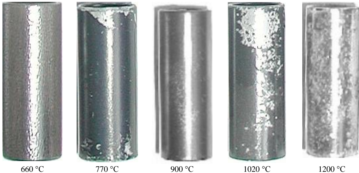
Fig. 3. Appearance of zirconium alloys samples after tests in a water vapor environment
