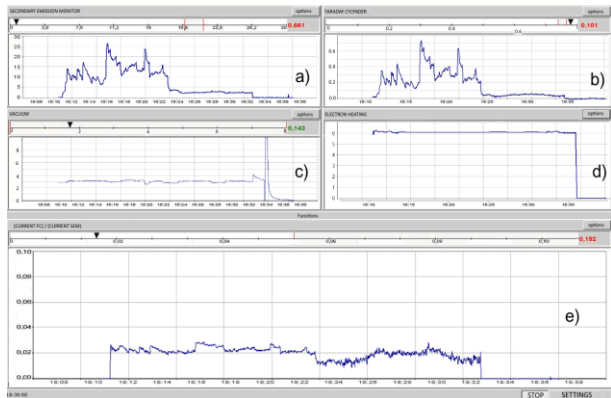
Fig. 14. The main window view of the M-30 microtron control panel: time dependence of the current of the SEM (a); current of the FC (b); signal of vacuumeter VIT-2 (c); the heating voltage of the cathode LaB_6 (d); the ratio (current of the FC) / (current of the SEM) (e)
