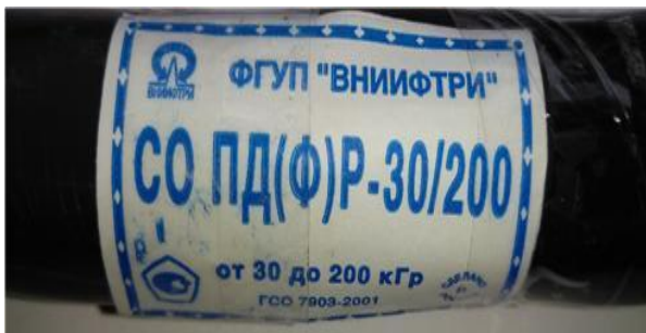
Fig. 1. Fragment of the arrangement of standard samples of the absorbed dose of electron radiation on the surface of the protective polymer jacket of the cable
