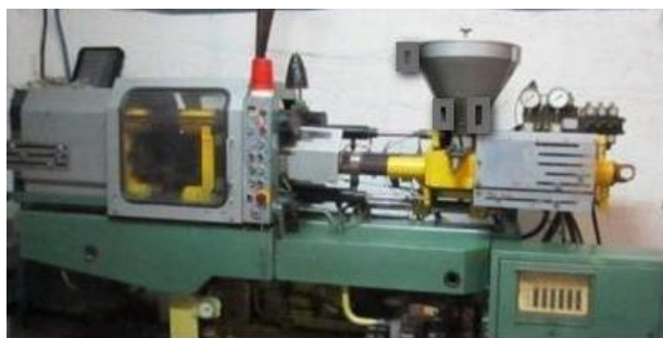
Fig. 1. Photograph of thermoplastic Windsor SP 80 with structural modifications
