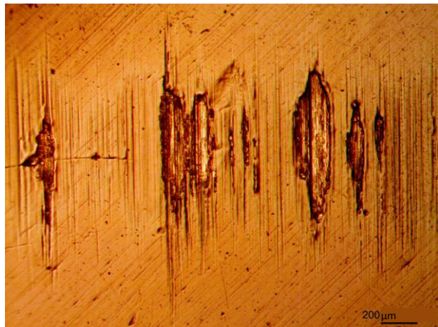
Fig. 3. Traces of abrasive wear on the surface of a three-layer DLC with a thickness of 2.4 μm
