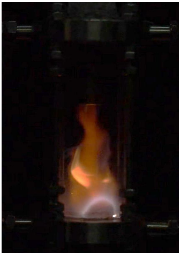
Fig. 2. Photograph of rotating gliding discharge at different operation modes (125 \mu s exposition): 10 l·min -1 airflow into discharge chamber, 5 l·min -1 airflow into reaction chamber, 0 g·min -1 ethanol flow (a); 10 l·min -1 airflow into discharge chamber, 5 l·min -1 air flow into reaction chamber, 8.5 g·min -1 ethanol flow (b)
