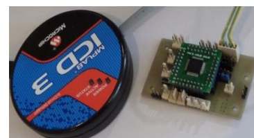
Fig. 5. Programmer and printed circuit board with microcontroller
