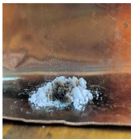
Fig. 4. \text{BaSO}_4 sample after laser irradiation
