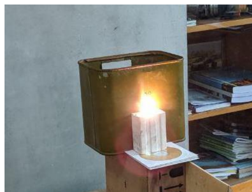
Fig. 3. \text{ZrO}_2 micropowder under laser beam effect
