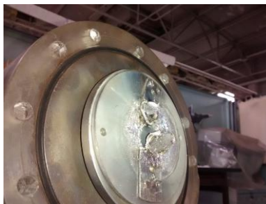
Fig. 2. Pucks after an irradiation
