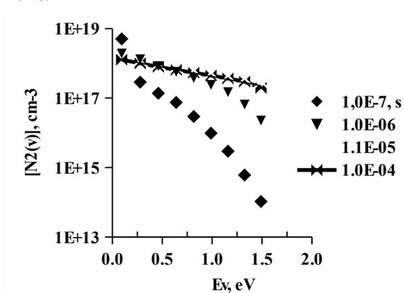
Fig. 1. Dependences of the concentrations of vibrational excited nitrogen molecules on the energy of vibrational excitation at various time exposures of gas in dry air plasma: 10<sup>-7</sup>, 10<sup>-6</sup>, 10<sup>-5</sup>, 10<sup>-4</sup> s
