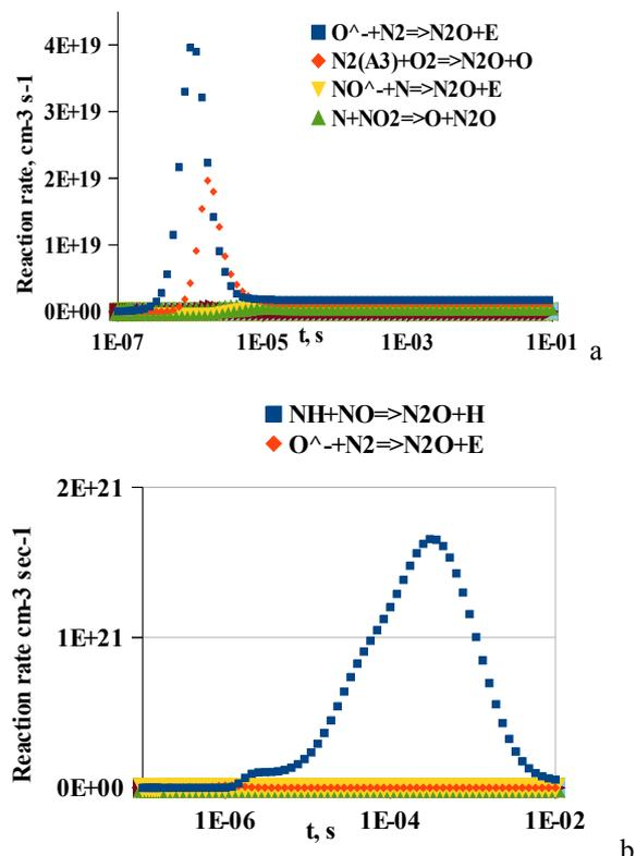
Fig. 4. Dependence of reaction rates which lead to the generation of  $N_2O$  from the exposure time of dry (a) and humid (b) air in plasma. At  $E = 1000 \text{ V cm}^{-1}$ ,  $T = 1000 \text{ K}$
