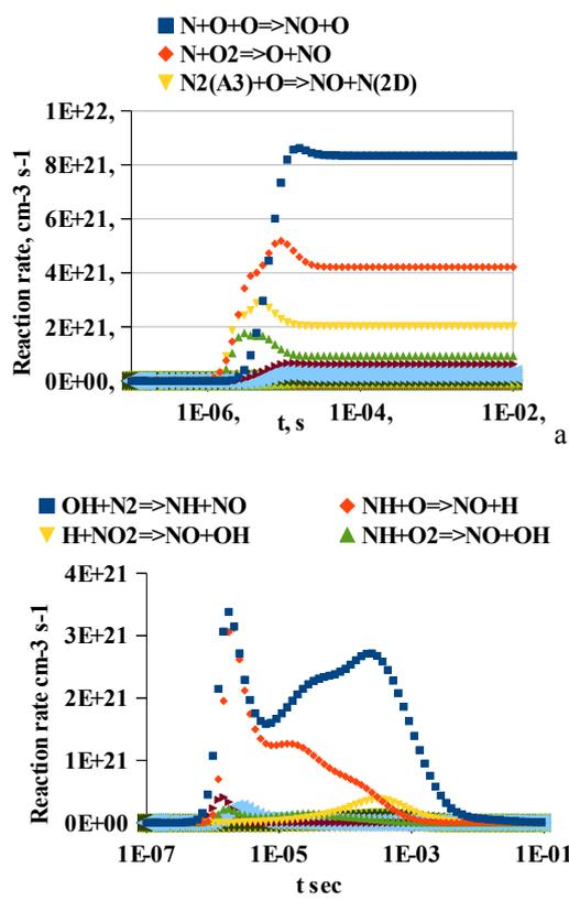
Fig. 3. Dependence of reaction rates which lead to the generation of NO from the exposure time in plasma of dry (a) and humid (b) air. At  $E = 1000 \text{ V cm}^{-1}$ ,  $T = 1000 \text{ K}$
