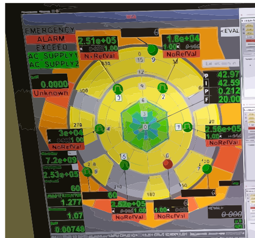
Fig.21. Typical neutron flux azimuthal distribution
