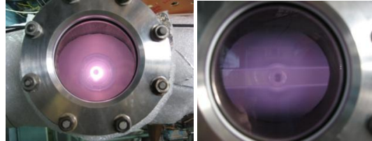
Fig. 3. The photo of high-frequency discharge created with the rod (left) and planar (right) antenna.
